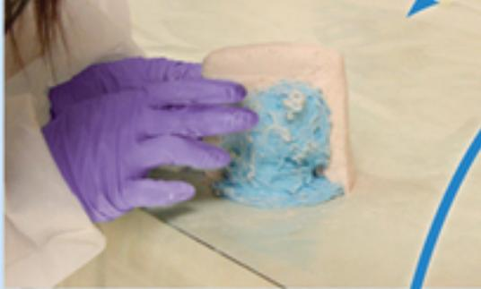
3. With the original part removed and mold secure, cast a new part. *Repro Fast-Cast Urethanes* are a popular choice for quick casting and demolding!
