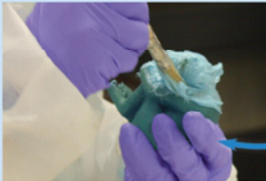
1. Create a flexible glove mold by brushing the silicone on the part, filling in all cracks and voids. It will easily peel away from the part but you now require a back-up so it can hold its shape during the casting process.
