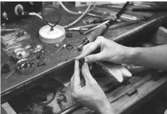
*Step 10: A wire wax is attached to the finished wax design to ready the piece for casting or to make a model.*
