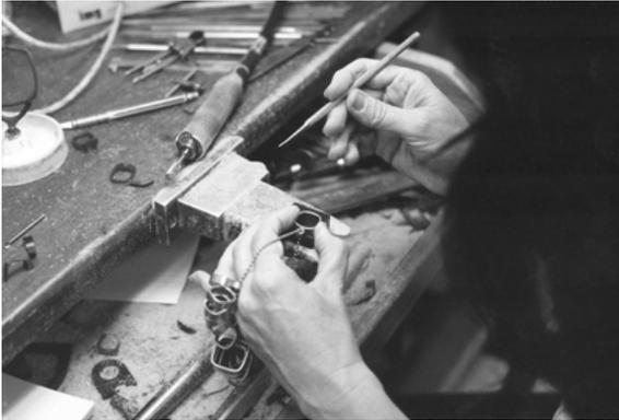
*Step 6: The hole is cut into the File-A-Wax piece using a motor tool. This can also be done with a carving knife.*
