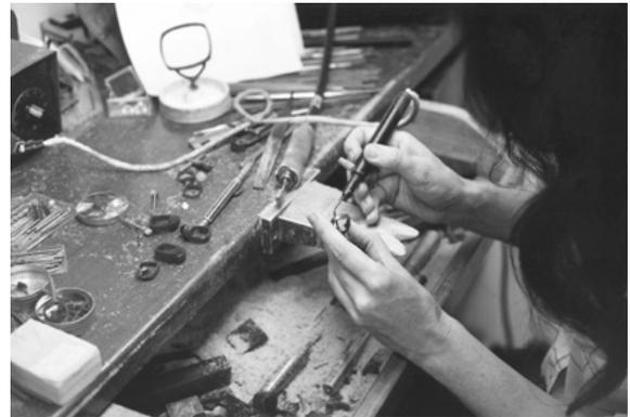
**Step 3:** *Filing down the Ring Tube segment creates the rough shape of the finished piece and readies the piece for design work.*
