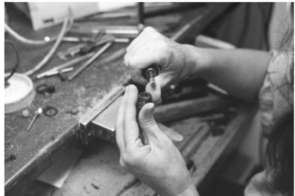
*Step 9: The stone is test fit in the bezel to check rough seating, positioning and overall design aesthetics.*
