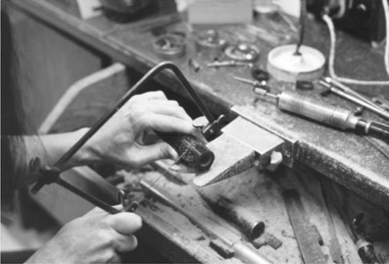
**Step 5:** *Attaching a wire wax to serve as a sprue is the final step before casting or creating a pattern.*
