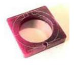
**Step 4:** Cut 3 square edged pieces of the hinge wax, making one piece 2 mm and the other two about 3 mm each. Slide the three pieces onto a drill shank, with the 2 mm. one in the center.
