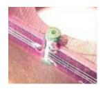
**Step 6:** Remove drill shank and file the outer hinge pieces flush with the sides of the bracelet.
